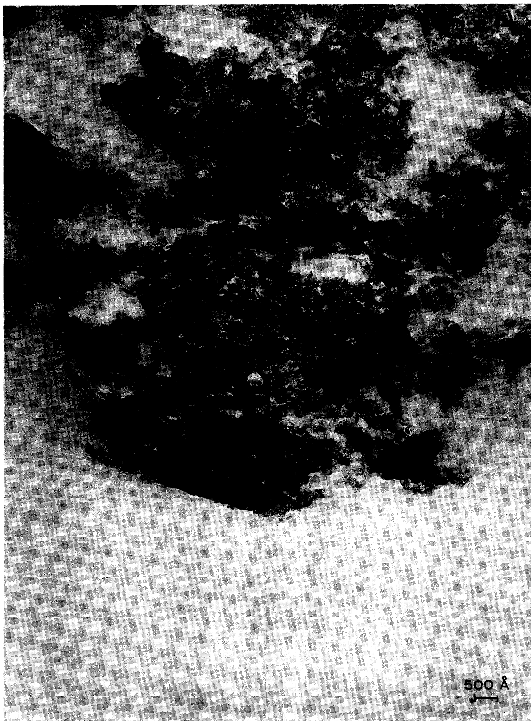
FIG. 2. Electron micrograph of a homogeneously precipitated nickel-on-silica catalyst. Nickel content: 35.4%; reduced at 370°C for 94 hr, evacuated at 370°C for 20 hr. Preparation of sample: see text. Enlargement: 140 000 \times (Siemens Elmiskop).
