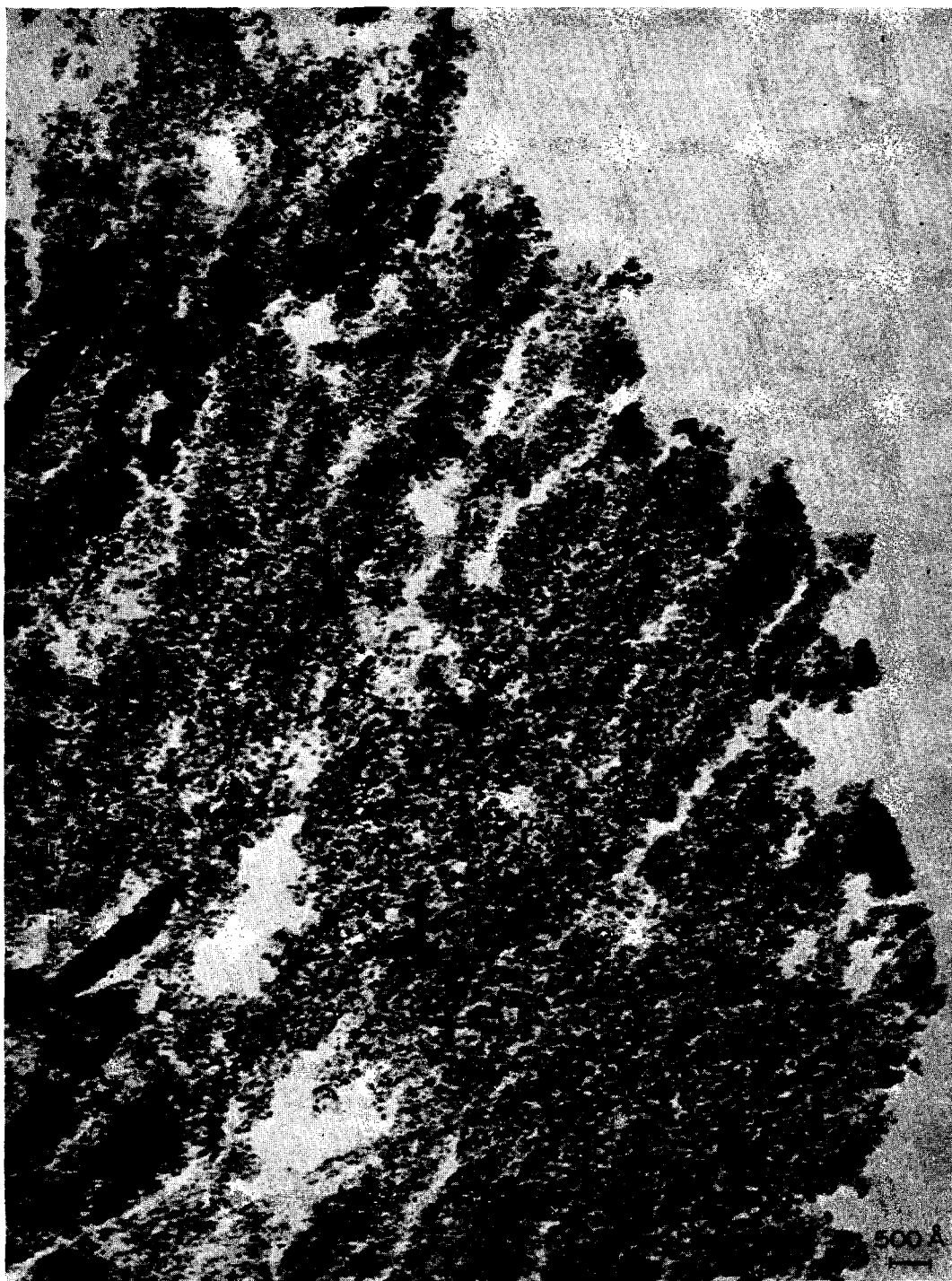
FIG. 3. Electron micrograph of nickel-on-silica catalyst. Harshaw Ni-0104 P (58.5% nickel); reduced at 310°C for 24 hr, evacuated at 290°C for 19 hr. Preparation of sample: see text. Enlargement: 140 000 \times (Siemens Elmiskop).
